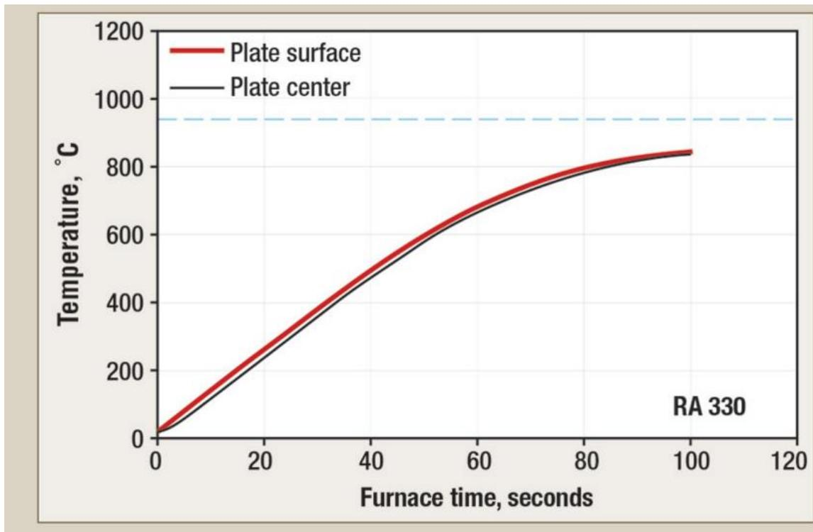
Fig. 1a. Calculated heating temperature profiles of the tray materials
